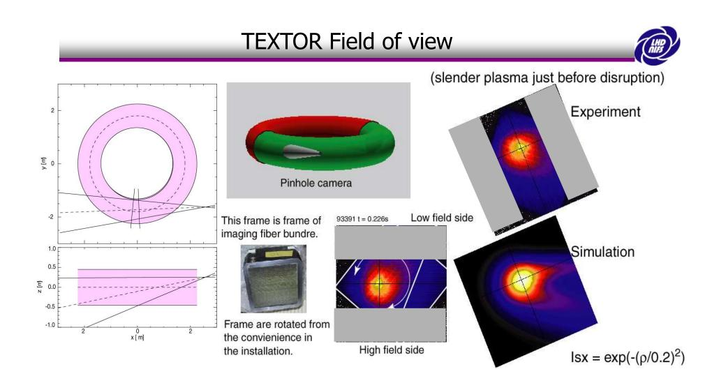
• Field of view is tilted. With old camera, it is also fairy narrow when we want to measure with higher framing rate, e.g. 9kHz.
